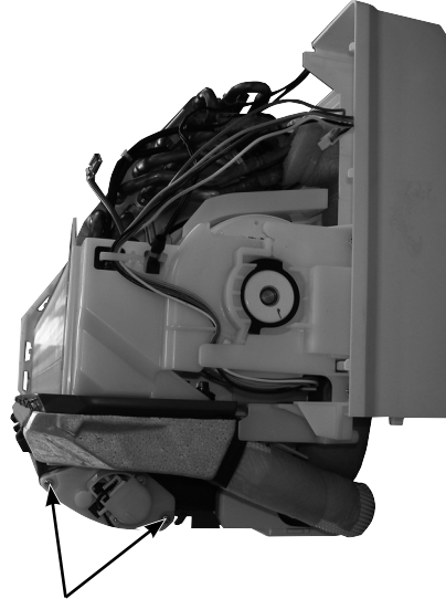
Screws of horizontal vane motor unit
